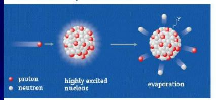
Spallation: A nuclear process in which a high energy proton excites a neutron rich nucleus which decays sending out neutrons (and other particles).
