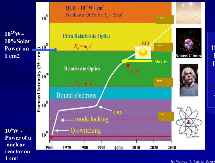
At focal point of the laser(microns)  $E = 9 \times 10^{6} MV/cm$ for an intensity of 10<sup>23</sup>W/cm2
